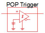
Periodic Operating Point (POP) Analysis in SIMPLIS is used to find the steady-state operating point of a converter
